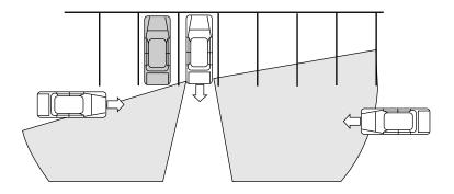
CTA coverage also decreases when parking at shallow angles (refer to figure for approximate zone coverage areas [sensor obstructed for vehicle on left]).
